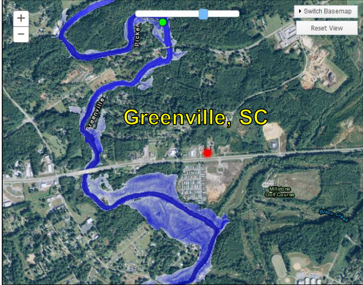
Inundation graphic for Greenville, SC based on crest of 12.0 feet
